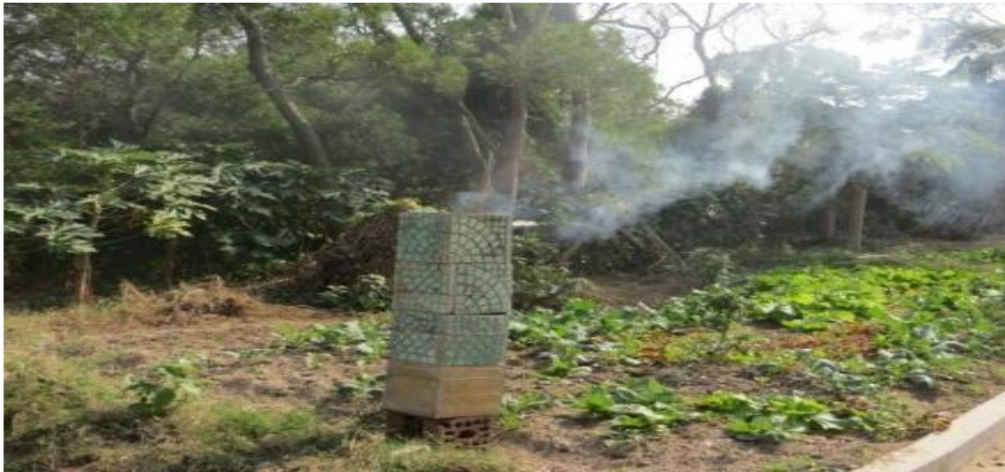
Fig. s1 the column-shaped stove
